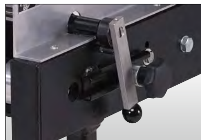
Simple adjustment of the separating gap.
