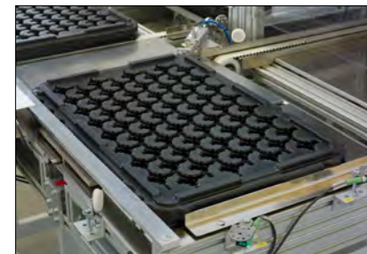
Filling position with pneumatic centering station.
