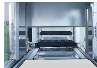
Linear conveyor section with stacker.
