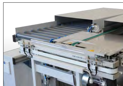
Filling position with package centring.
